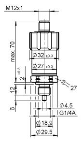
Probe length Probe diameter 6 mm 4.5 mm 50 mm 8 mm 100 mm 8 mm 250 mm 8 mm 350 mm 8 mm
