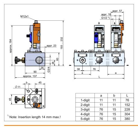
Cable socket M12 with screw terminals in the scope of delivery
