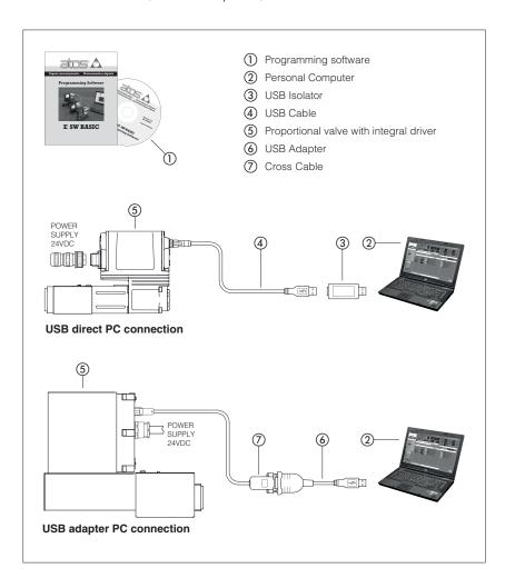
The E-SW / Z-SW programming software are the entry door to the Atos digital technology. They are supplied in DVD format and can be easily installed on a desktop or a notebook computer.
