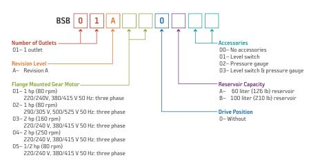
The BS-B Lubricator features a smart part number ordering system, where you can tailor the pump to meet your needs. First, choose the number of outlets, revision level, flange mounted gear motor, drive position, reservoir capacity and accessories you need. Then, put the numbers into the corresponding squares in the easy-to-use grid. You now have the customized part number.
